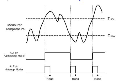
Figure 2. ALT Pin Modes of Operation
