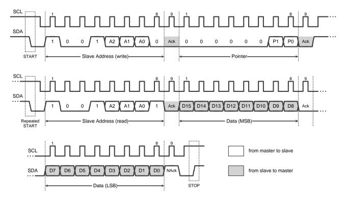
Figure 5. Two-wire Read Command Timing Diagram
