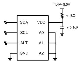
Figure 6. Typical Connections of the GD30TS076C
