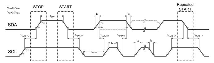
Figure 3. Two-Wire Timing Diagram
