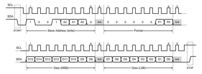
Figure 4. Two-wire Write Command Timing Diagram
